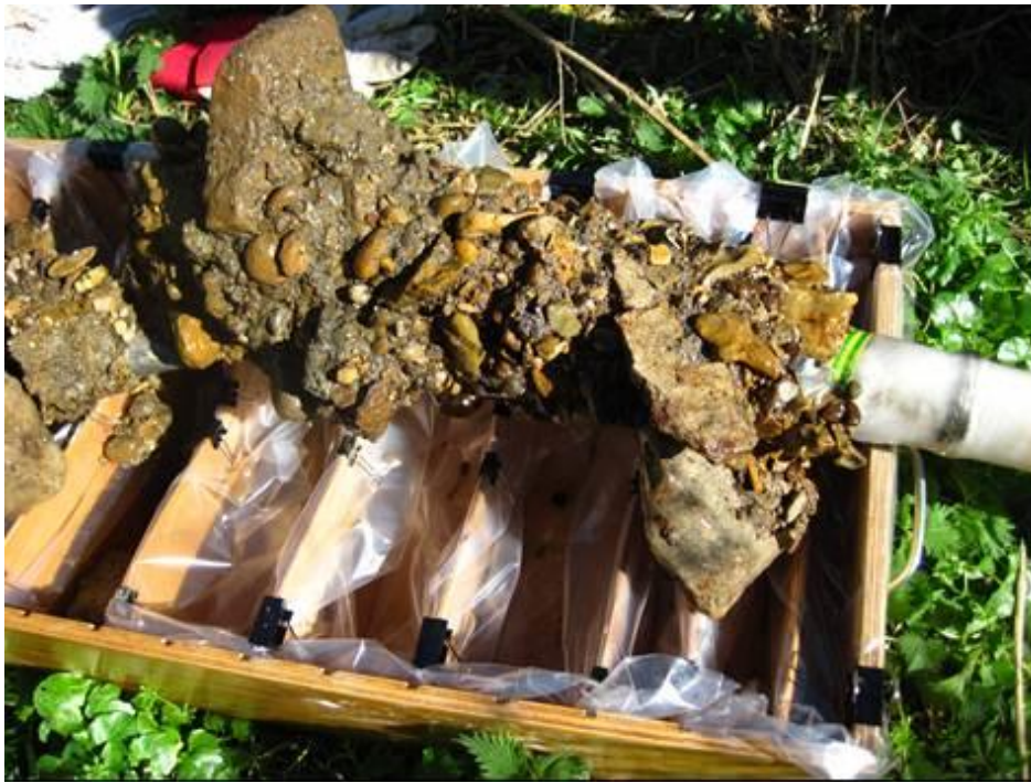
Figure 5.26. Freeze core sample (gravel jetted) over segmentation box, Pinchmill.
