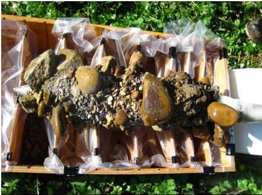
Figure 5.24. Freeze core sample over segmentation box, Pinchmill.
