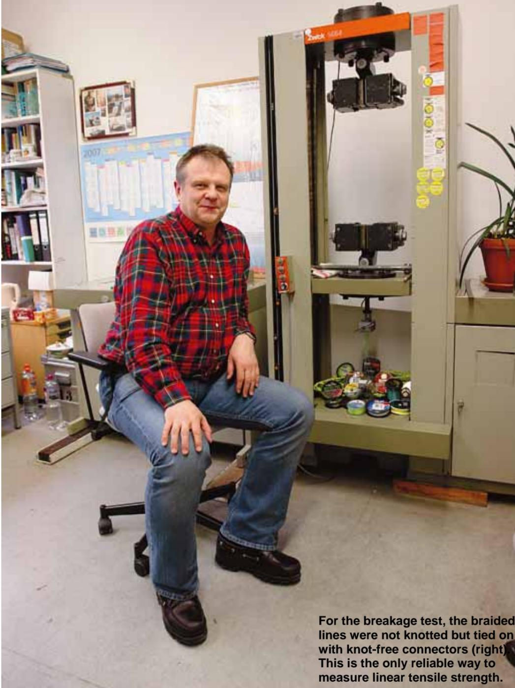
For the breakage test, the braided lines were not knotted but tied on with knot-free connectors (right). This is the only reliable way to measure linear tensile strength.
