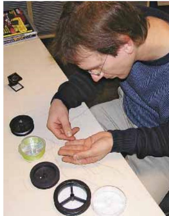
In the blind test, the surface, suppleness and braiding were examined and compared – with surprising results: lines with similar manufacturers' details exhibited significant differences.
